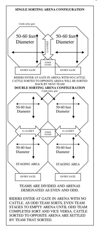
The optimum sorting pen is 50'-60' diameter with corners cut at 45'.
