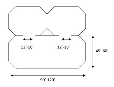
a) Three man two gate sorting will take place in a pen that is 90 to 120 foot in size. There will be two 12' to 16' gates on one side of the pen.
