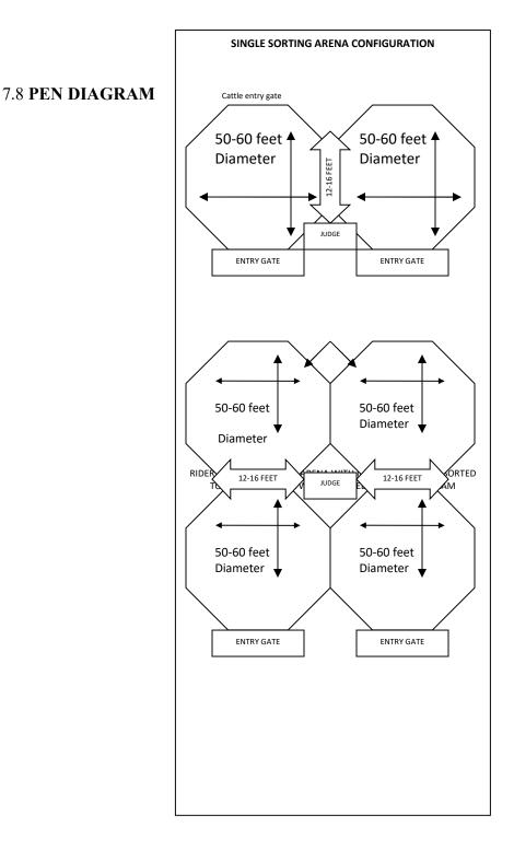
The optimum sorting pen is 50'-60' diameter with corners cut at 45'. The opening between the two pens will be 12'-16'.
